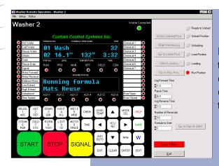
Manual screens, like this one for washer controls, make it easy to control the system for test and maintenance.
