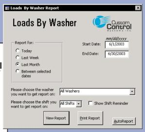
Washdeck production reports give you a picture of the efficiency of your plant. Additional reports show machine faults and formula run time and machine turnaround time.
